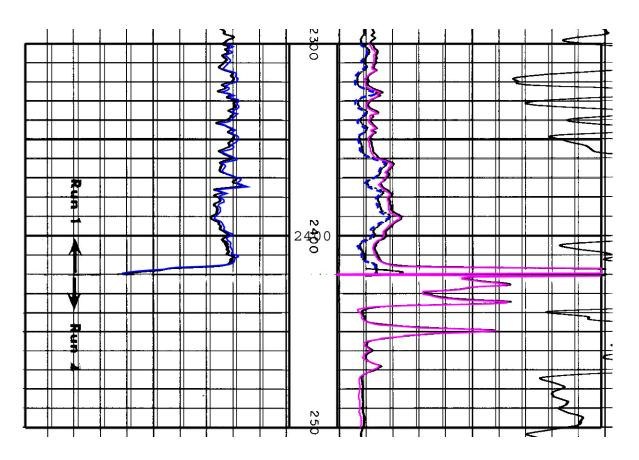
IES to 2420' has solid line coding for SN and dashed for induction. Below 2420, a single induction log was run in oil-base mud with solid line coding. The logs were then spliced together. The digitizer followed the solid line coding and captured the induction below 2420' as part of the SN curve.
